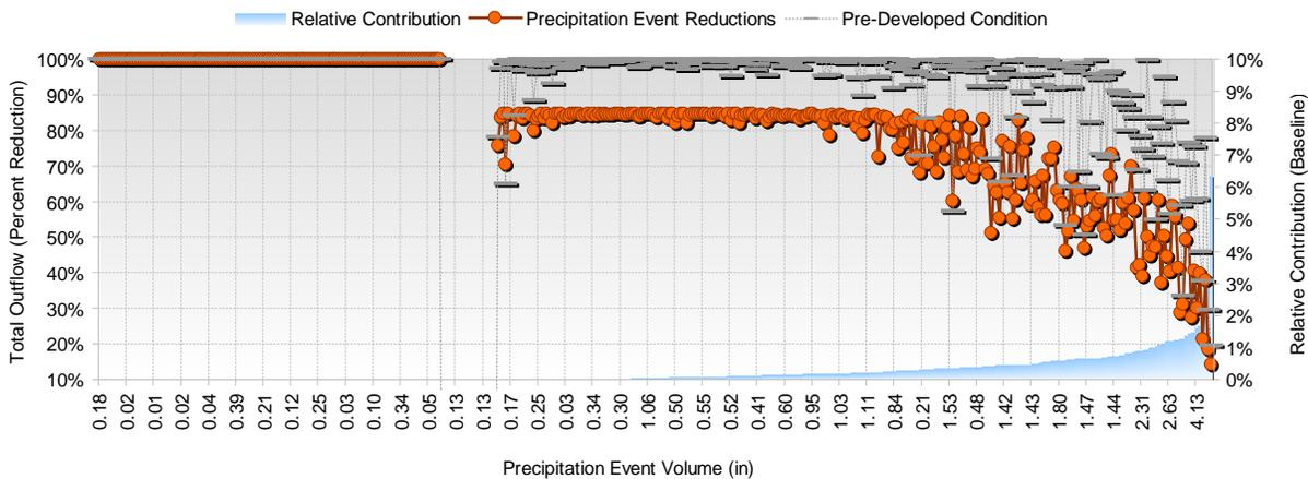
Figure 3-23. Solution 1 Flow Volume Reduction Effectiveness by Storm Events.
