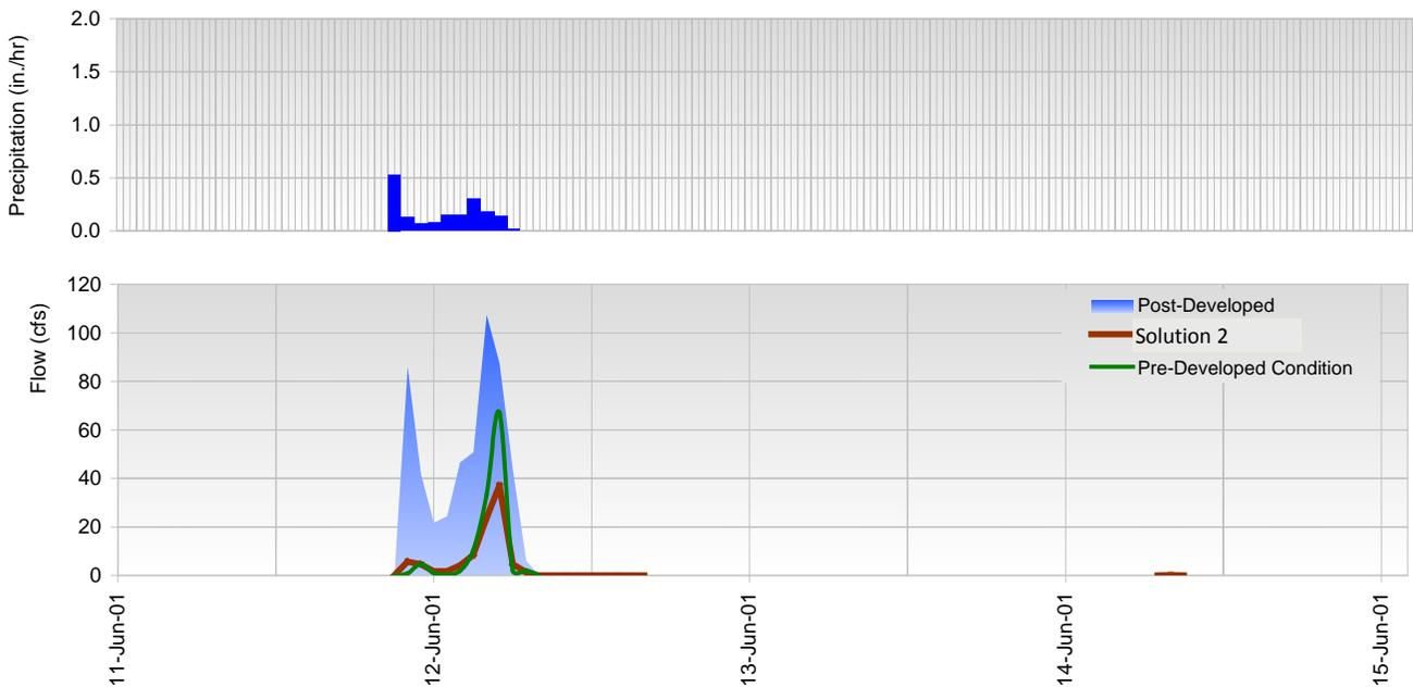
Figure 3-27. Solution 2 Hydrograph for the June 2001 Storm Event.
