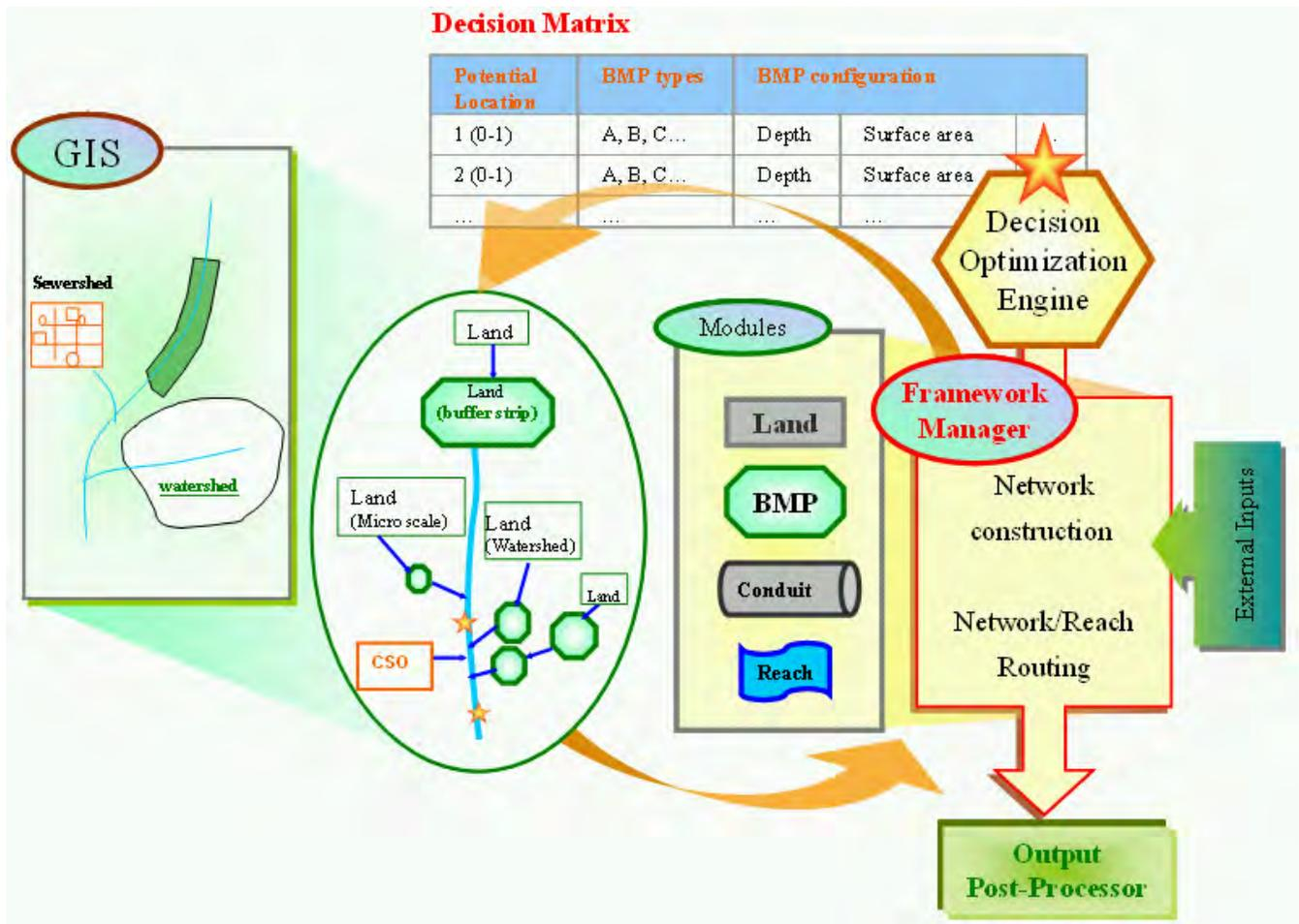
Figure 3-2. SUSTAIN Components and Flow Chart.
