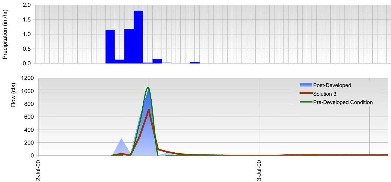
Figure 3-30. Solution 3 Hydrograph for the July 2000 Storm Event.
