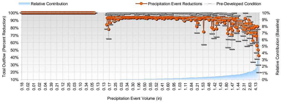
Figure 3-24. Solution 2 Flow Volume Reduction Effectiveness by Storm Events.
