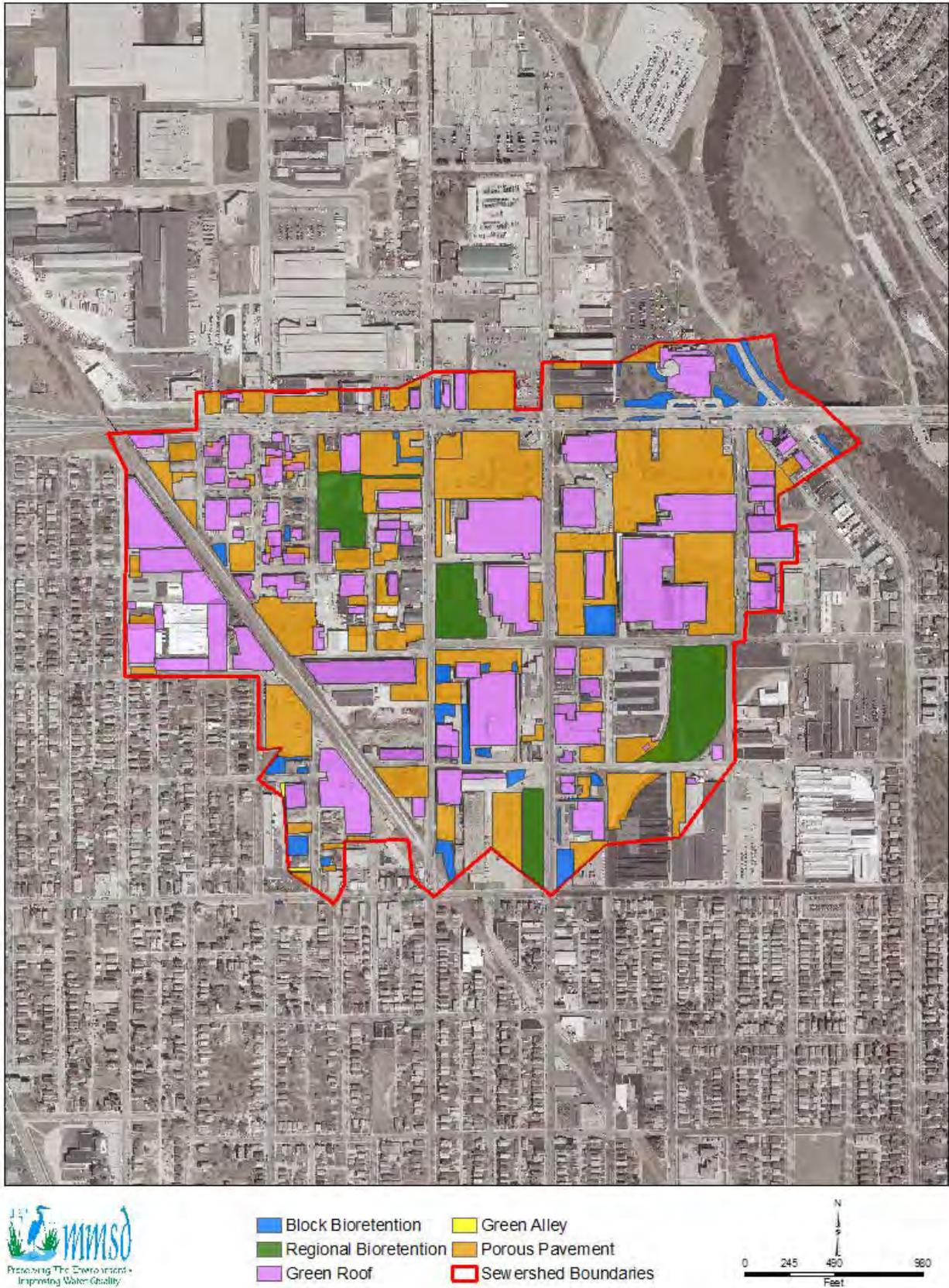
Figure 3-8 to Figure 3-11 for each of the four sewerheds. Rain gardens, rain barrels, green alleys, and roadside porous pavement were not mapped spatially. Table 3-6 summarizes the maximum extent of each practice in each
