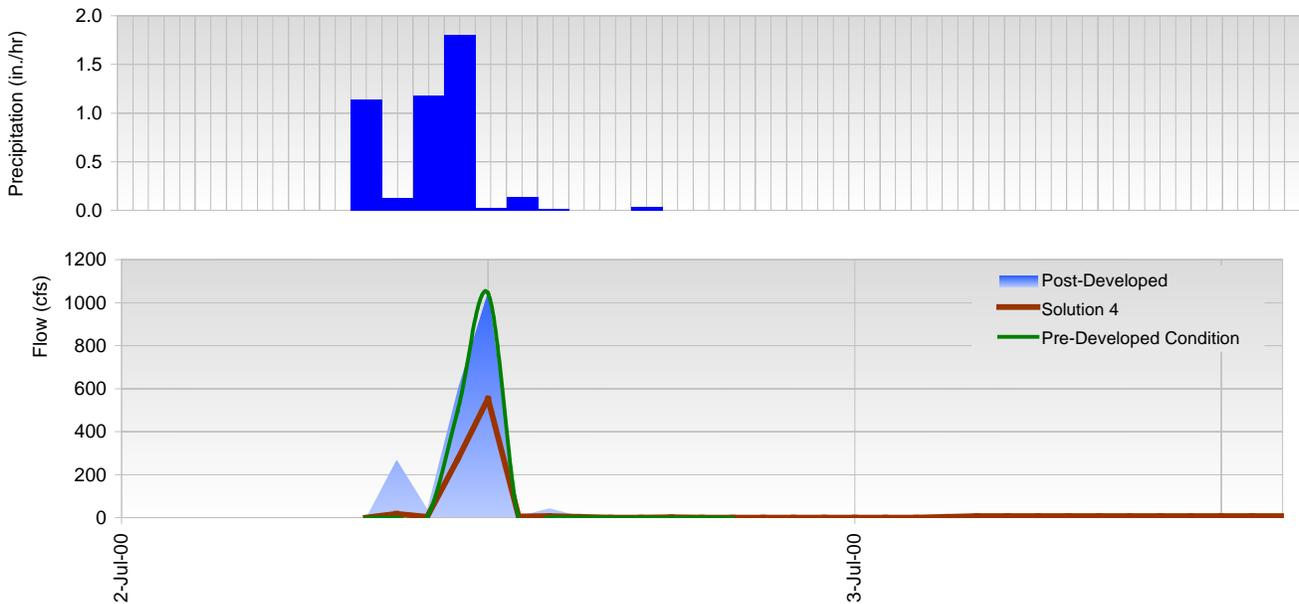
Figure 3-31. Solution 4 Hydrograph for the July 2000 Storm Event.
