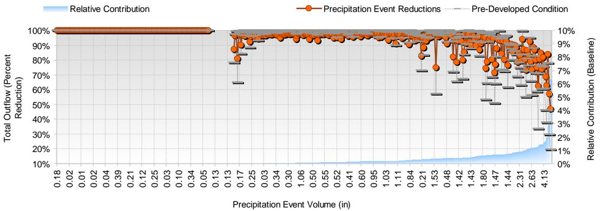
Figure 3-26. Solution 4 Flow Volume Reduction Effectiveness by Storm Events.
