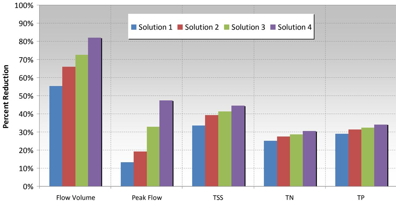
Figure 3-32. Flow Volume, Peak Flow, and Pollutant Loading Reductions of the Four Selected Solutions.
