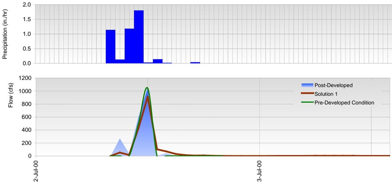
Figure 3-28. Solution 1 Hydrograph for the July 2000 Storm Event.
