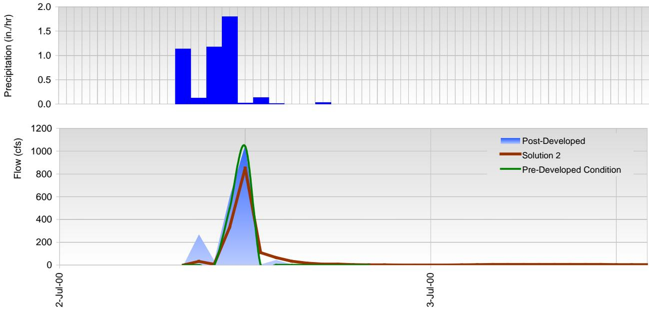
Figure 3-29. Solution 2 Hydrograph for the July 2000 Storm Event.
