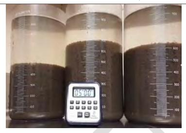
FIGURE 6E-2: GRANULAR SLUDGE AFTER 5 MINUTES SETTLING
