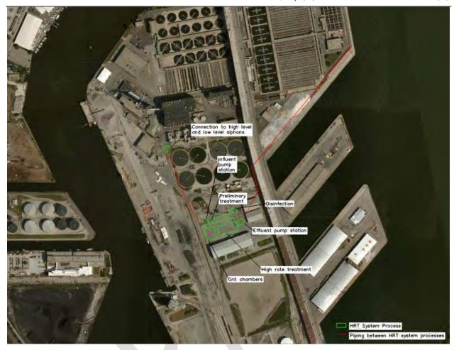
FIGURE 6E-9: JIWRF HRT SYSTEM LAYOUT
