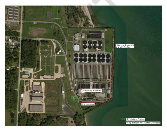
FIGURE 6E-10: SSWRF HRT SYSTEM LAYOUT
