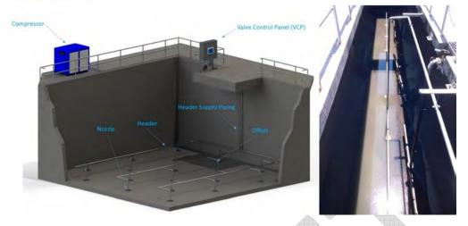
Figure 3: Standard Layouts for Large Bubble Compressed Air Mixing System
