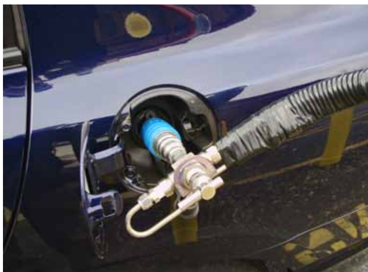
MMSD Natural Gas Vehicle Fueling
