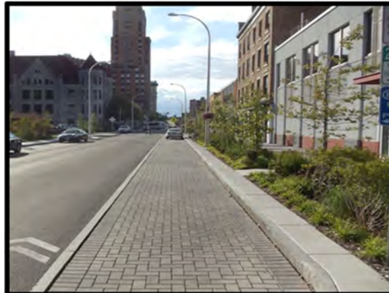
Porous paver parking lane with bioretention garden.
