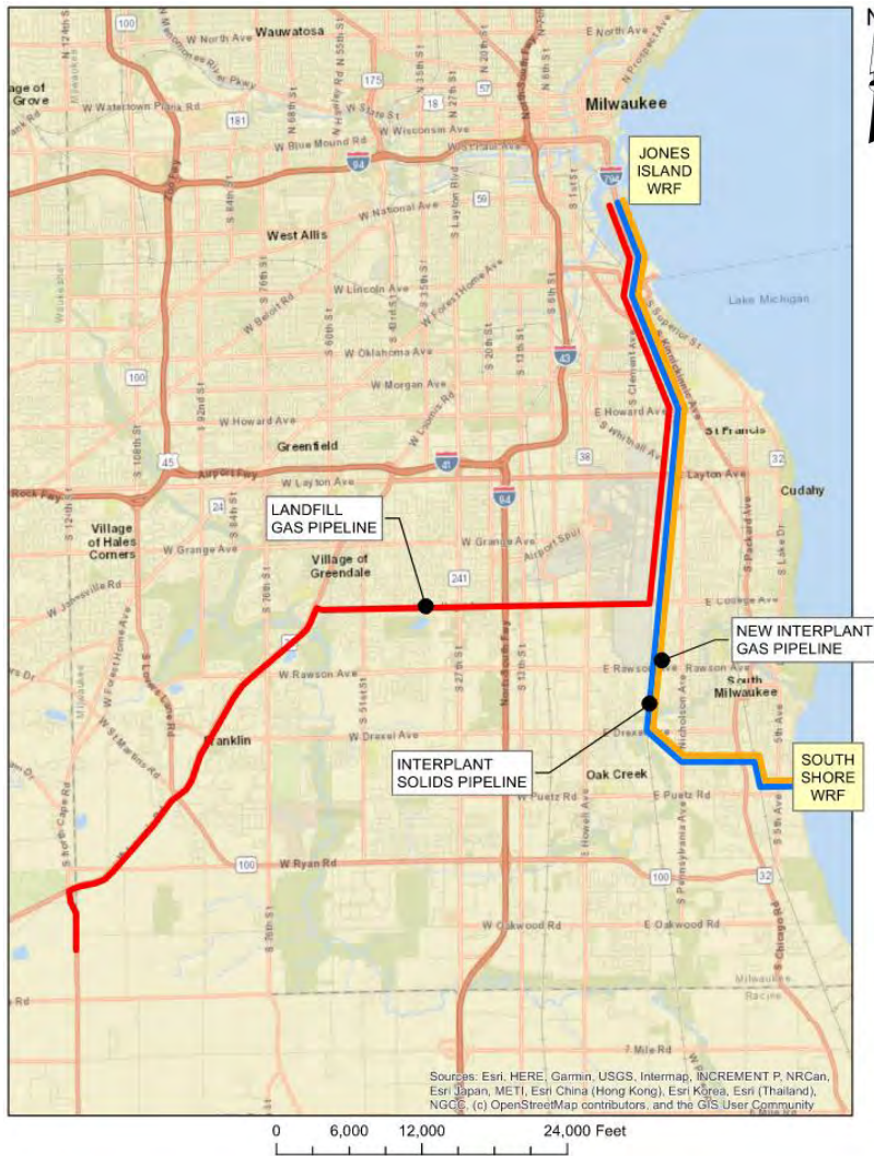
Figure 4-5: SSWRF to JIWRF DG Pipeline
