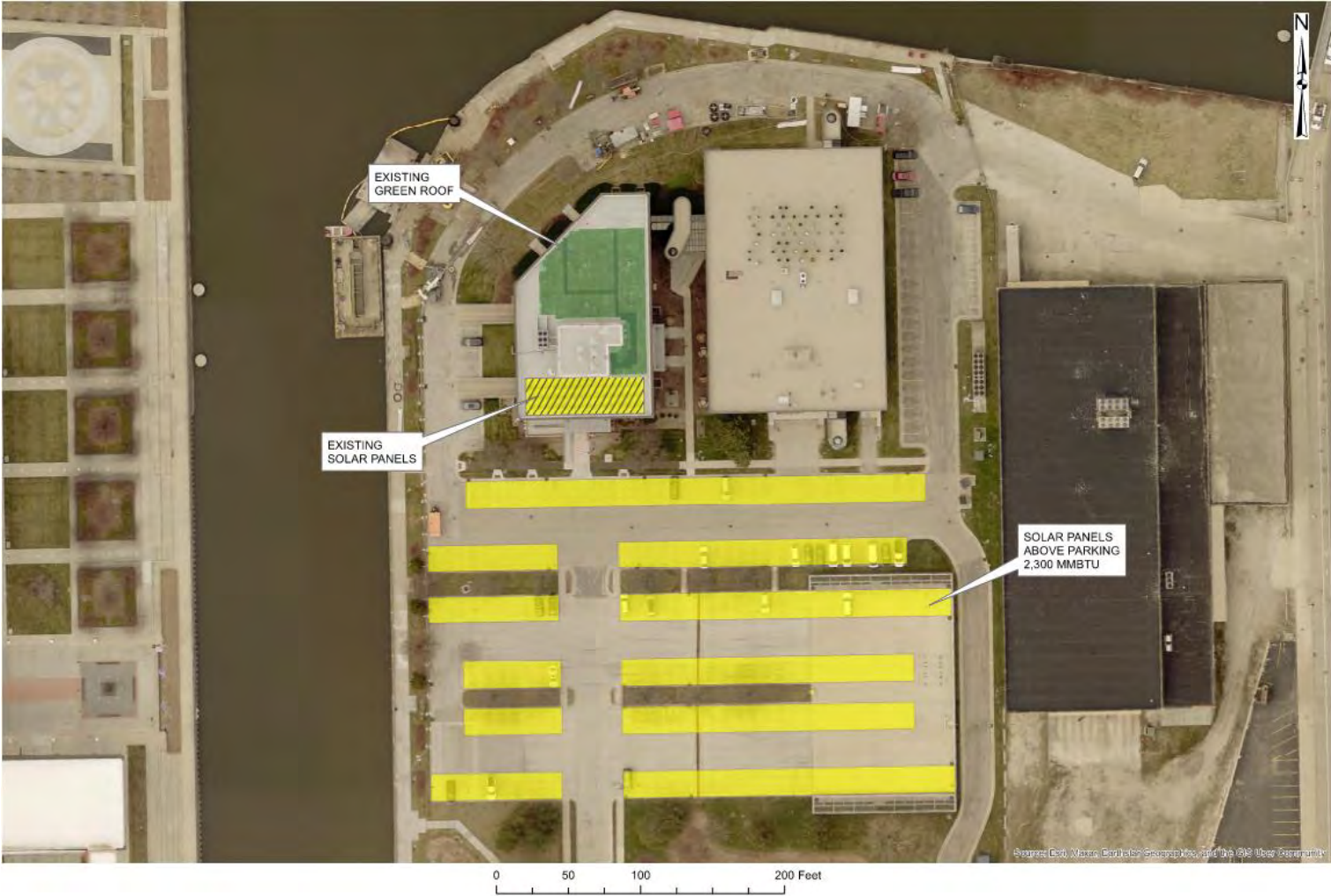
Figure 4-6: Administration Facilities Recommended PV Locations
