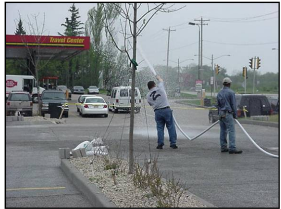
Figure 16. Testing pervious concrete with a fire hose.
