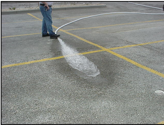
Figure 15. Water discharged from a fire hose quickly infiltrates the pervious concrete.
