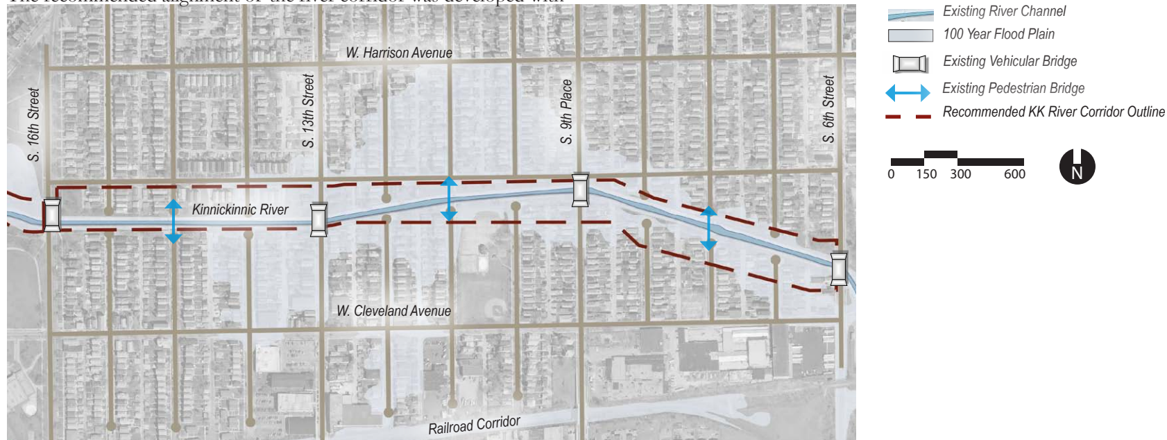
Figure 3-2. Approximate limits of new river corridor alignment superimposed over existing orthophoto, S. 6th to S. 16th Streets
