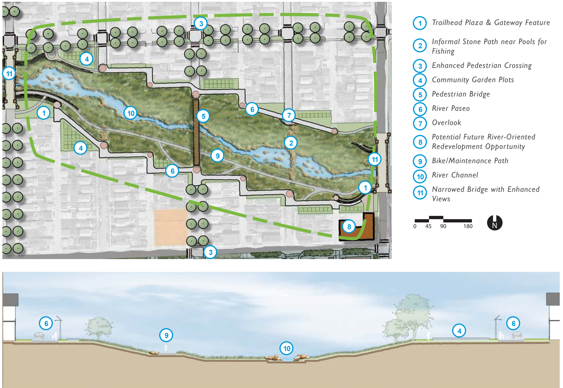
Figure 3-6. “Grow” (S. 6th St to S. 9th Pl) plan view and typical cross-section
