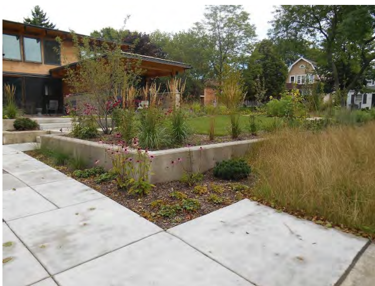
GI captures stormwater and allows it to soak into the ground or evaporate instead of running into watercourses or entering sewers and contributing to sewer overflows. Photo credit: MMSD
