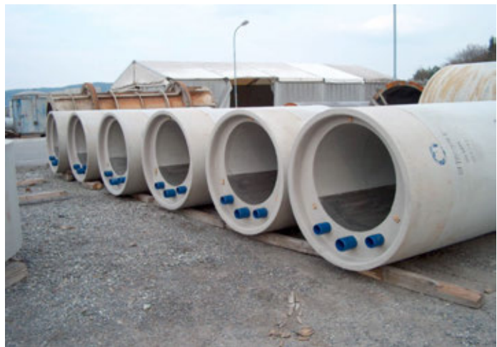
Integral heat exchanger for new sewers
