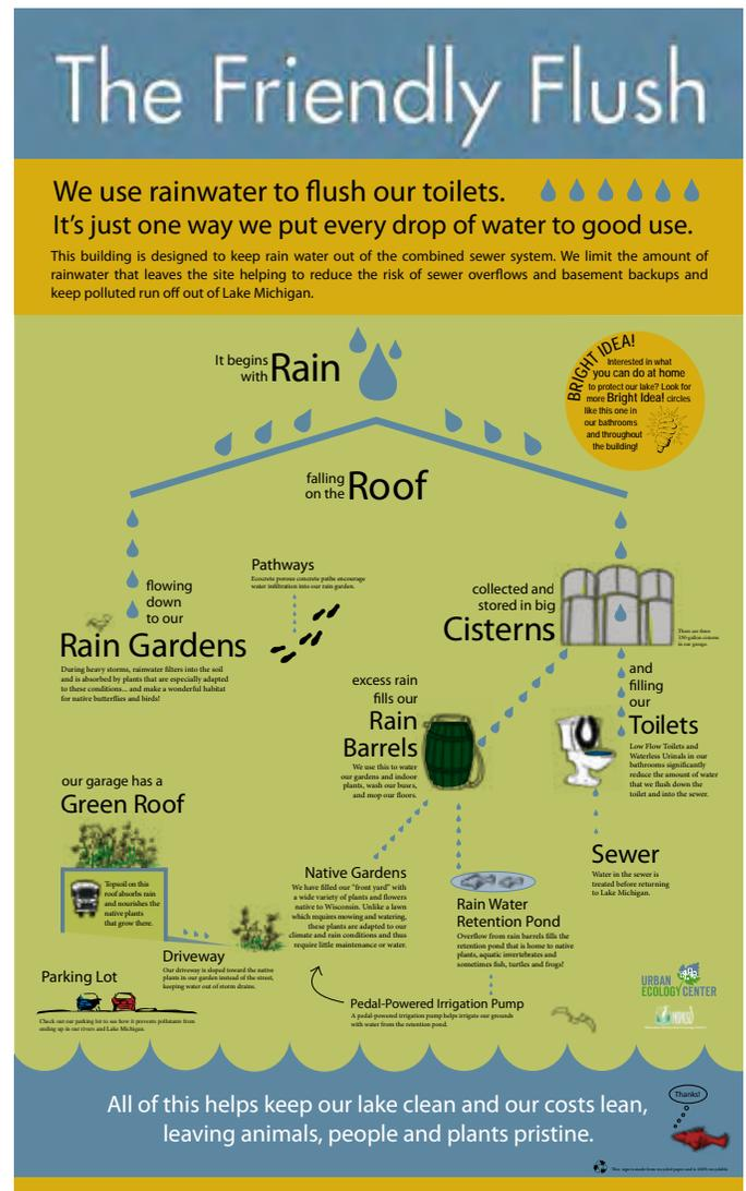
The Urban Ecology Center implemented a rainwater harvesting facility to water plants and flush toilets. Meeting the plumbing code to use rainwater to flush toilets led to many monitoring requirements that are not practical for expanded rainwater harvesting in the region. Working with the state on plumbing code changes to streamline the regulatory process will be important to expanding rainwater harvesting in the region. Image courtesy of the Urban Ecology Center
